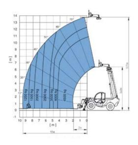
Lift capacity chart (with stabilisers)
